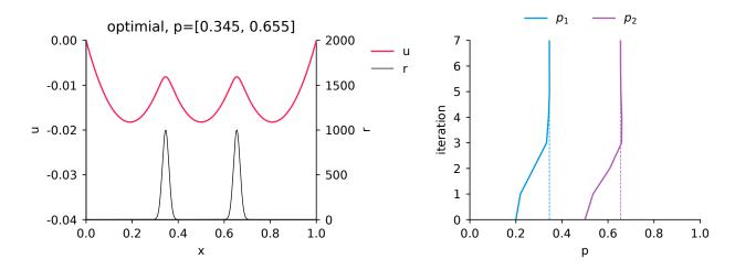
The pillars move to positions symmetric with respect to the center, and the average height of the bridge increases.
