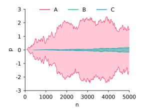
The thick solid lines show the envelope of the signal defined by its minima and maxima. The maximum achieved absolute values of the pressure are
